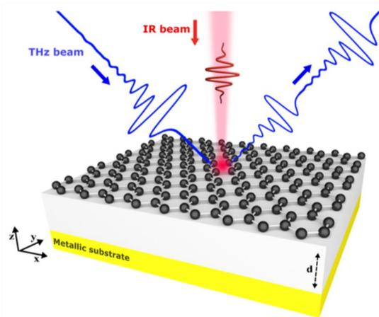
**Stimuli:** Optical pump by an amplified kHz Ti:Sapphire laser system, delivering 35 fs pulses at 800 nm and maximum energy of 2.3 mJ/pulse.
